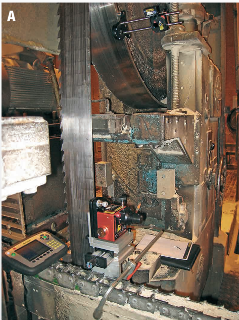
A. The rigid laser transmitter bracket allows for easy indexing (90°) to the band wheel. The wheels are aligned 90° to the centre line chain. The laser makes a constant sweep parallel to the wheel, which means you just place the detector anywhere within the laser sector and read off the value.
