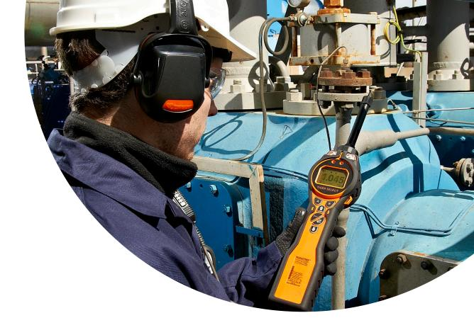
A revolutionary hand-held detector, Tiger Select can be operated either without a benzene pre-filter tube to detect total aromatic compounds (TAC) or with a benzene pre-filter tube to detect benzene selectively. For simplicity and ease of use, the Tiger Select has been split into two, user-friendly modes: Basic and Advanced. Both modes are user-selectable.
