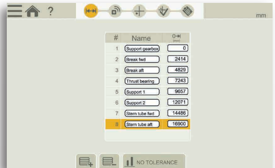
Bore center program, with bores individually named. If required, you can set tolerances.
